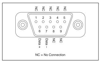
Figure 5. Dsub Connector Pinout
